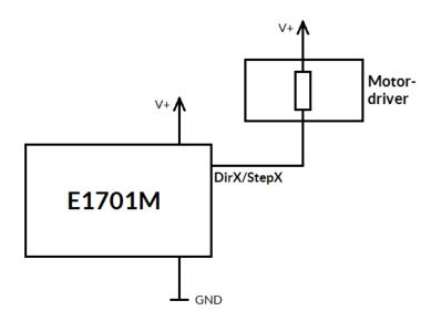
Here "DirX/StepX" symbolises one of the step- or direction outputs, V+ is either V (5V internal, non-insulated mode with both jumpers set) or  $V_{\rm ext}$  (up to 24V external, insulated mode with both jumpers removed). GND is either GND (non-insulated mode) or GND<sub>ext</sub> (insulated mode). The internal resistor of the connected device is not allowed to have less than 490 Ohms in order to not exceed the given current limits.
