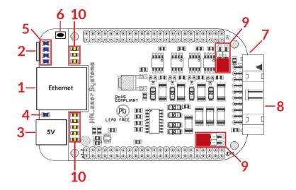
The E1701M motion controller board provides following connectors and interfaces:
